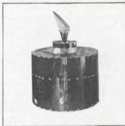
INTELSAT III satellite—56 inches in diameter, 41 inches high; 335 pounds in orbit; 1,200-circuit capacity; in use today in global system.
