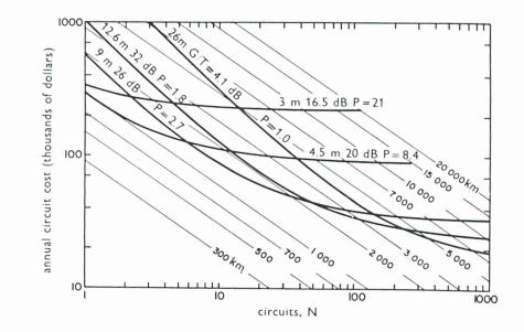
station has higher costs, even for a single circuit. Of course, a further 10 dB increase in the satellite EIRP would give even this 3 m station the advantage of bandwidth-limited operation; reducing all the (inferred) penalty factors as well. However, one should recognize the "cost" of this 10 dB, either in satellite power and weight, or in the shortening of routes within the narrower earthward beam.
