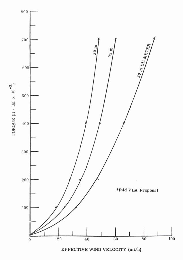
Figure 2-21. Torque Requirements Versus Wind Velocity For Different Size Reflectors\*
