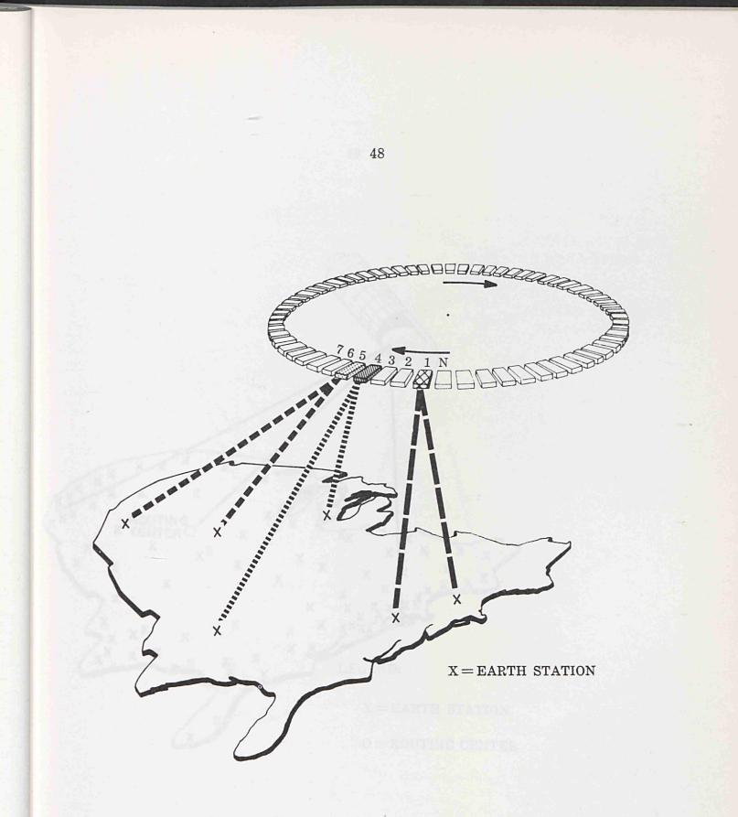
Figure 7. Time Slots (Channels) 1, 4, and 5 Have Been Temporarily Assigned to Connections Between the Earth Stations Illustrated. Channel 1 Connects New York City and Washington, D.C.; Channel 4 Connects Chicago and Dallas; and Channel 5 Connects Los Angeles and Denver
