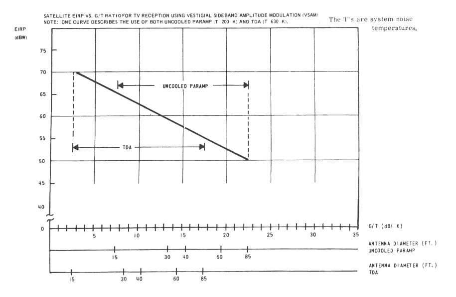
Figure 2-1. EIRP Versus G/T-VSAM @ 850 MHz,  $(S/N)_{o} = 53 \text{ dB}$
