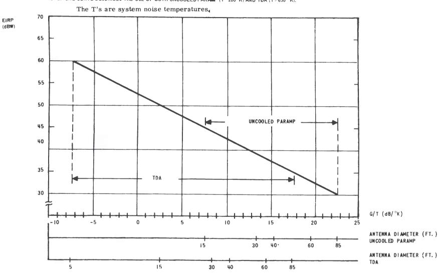
SATELLITE EIRP VS. G/T RATIO FOR TV RECEPTION USING VESTIGIAL SIDEBAND AMPLITUDE MODULATION (VSAM) NOTE: ONE CURVE DESCRIBES THE USE OF BOTH UNCOOLED PARAMP (T  $200^{\circ}$  K) AND TDA (T = 630° K).
