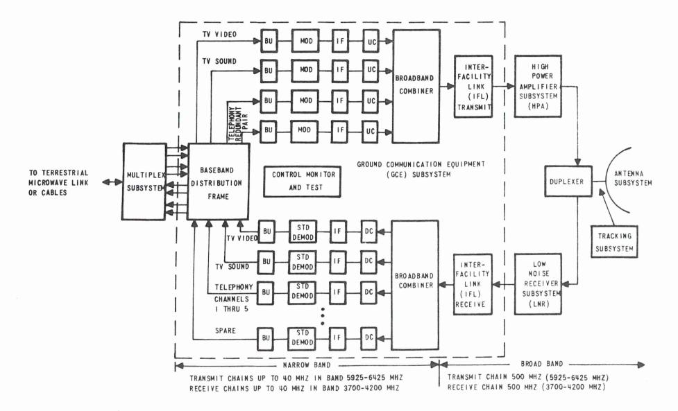
Figure 2-18. Satellite Communications Earth Station (Standard)
