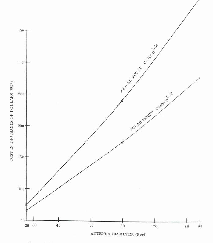
Figure 2-24. D. S. Kennedy Mesh Surface Steerable Antenna F.O.B. Factory Costs With Electric Drive and Front-Fed Feed
