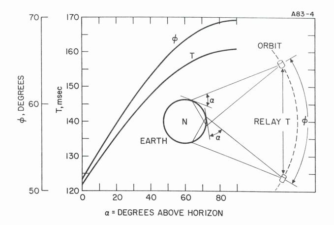
Fig. 2. Relay angle  $\varphi$  and additional time T as functions of elevation  $\alpha$  to the satellite.
