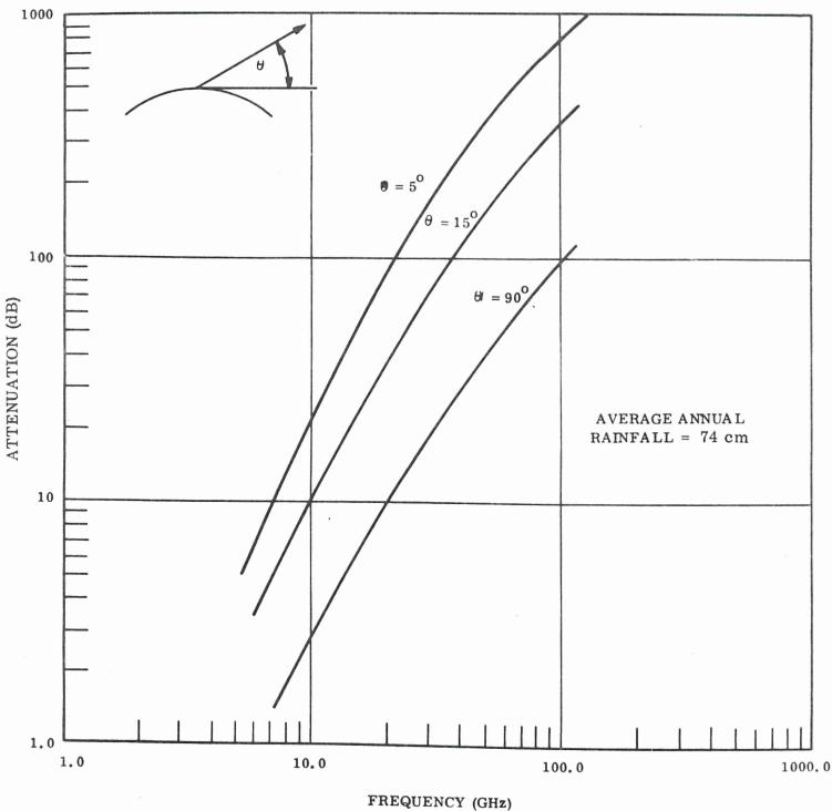
Figure 2-28. Rain Attenuation Versus Frequency
