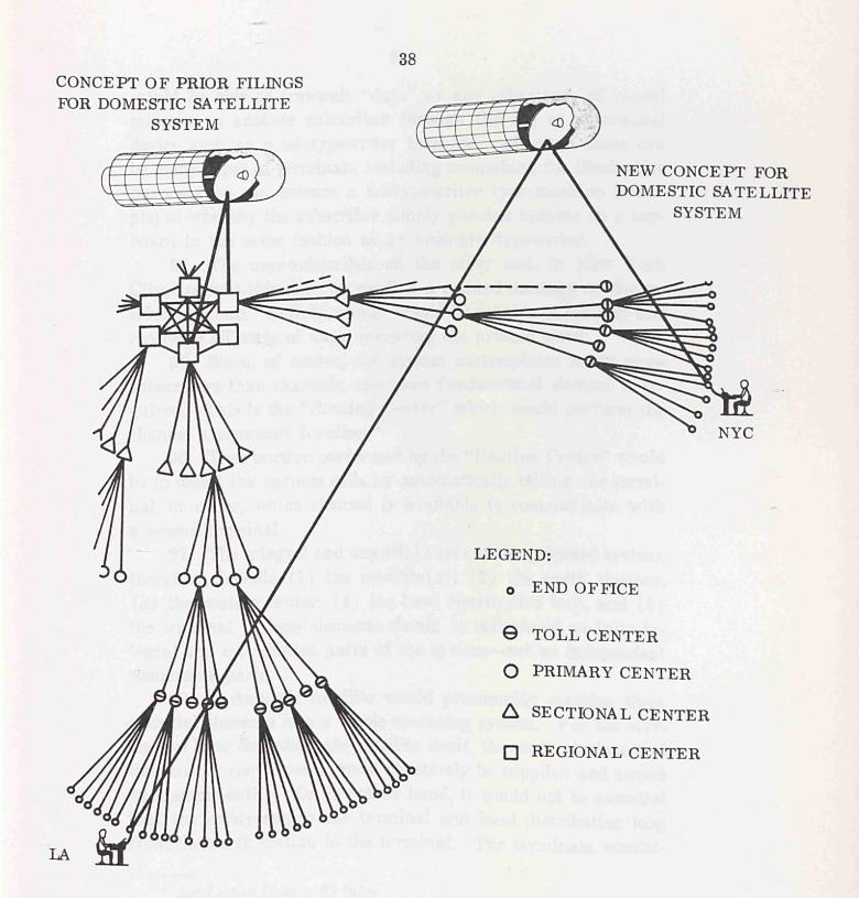
Figure 3. A Graphic Representation of the Difference Between the Prior Filings (Which Eliminate No Switching Centers) and the New Concept (Which Eliminates All Switching Centers Except the End Office)
