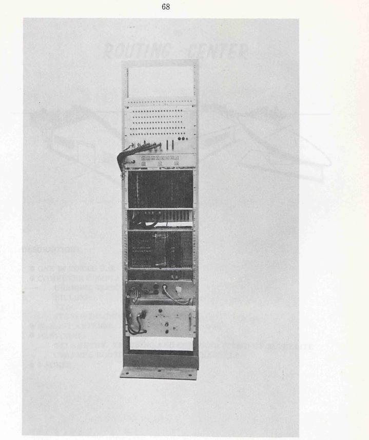
Figure 14. Multiple Access Digital Service (MADS) Automatic Digital Exchange (ADX) Development Unit
