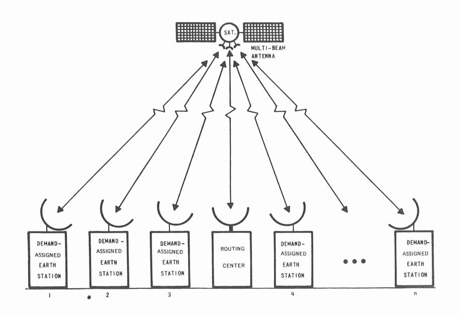
Figure 2-15. Block Diagram of Demand-Assigned Communications System
