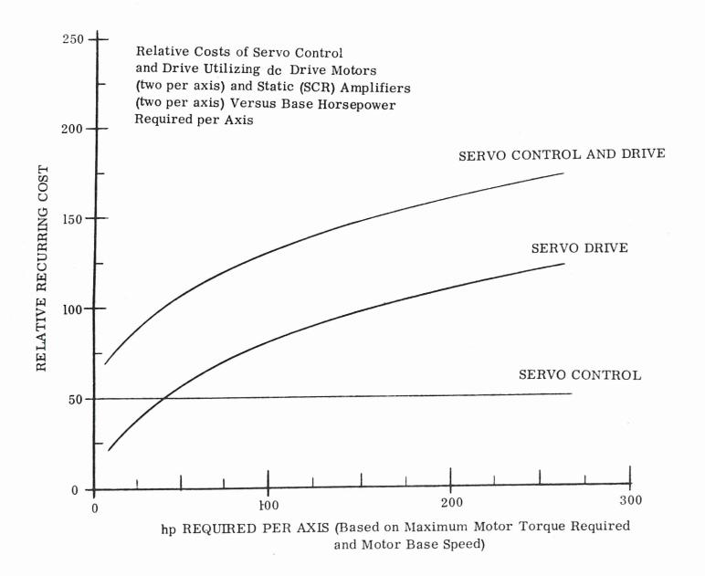
Figure 2-22. Relative Cost of Servo Drive Systems Versus Power Requirements
