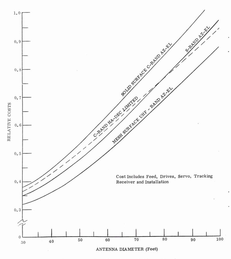
Figure 2-23. Steerable Antenna Costs Versus Diameter
