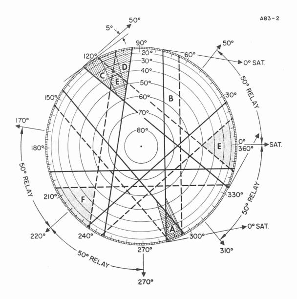
Fig. 3. Polar routing diagram for 5° to 15° elevation to satellites and relaying ±50° or less.
