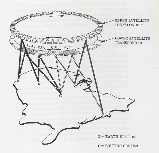
Figure 9. The Lower Transponder is Used on a Fixed Assigned Basis for Conversation Between the Earth Stations and the Routing Center. The Upper Transponder is Used On a Demand Assigned Basis For Traffic Channels Between Earth Stations
