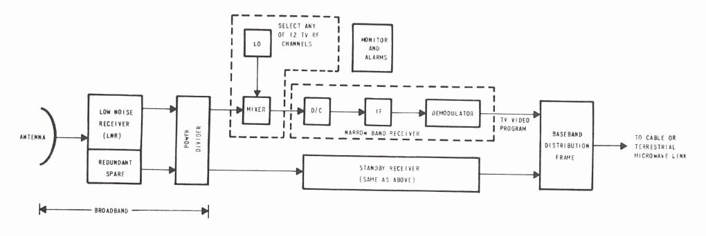
NOTE: D/C IS DOWN-CONVERTER WITH LO. IF IS IF AMPLIFIER AND FILTER. SPARE (STANDBY) EQUIPMENT CAN BE SWITCHED IN AND OUT 30TH MANUALLY AND AUTOMATICALLY.
