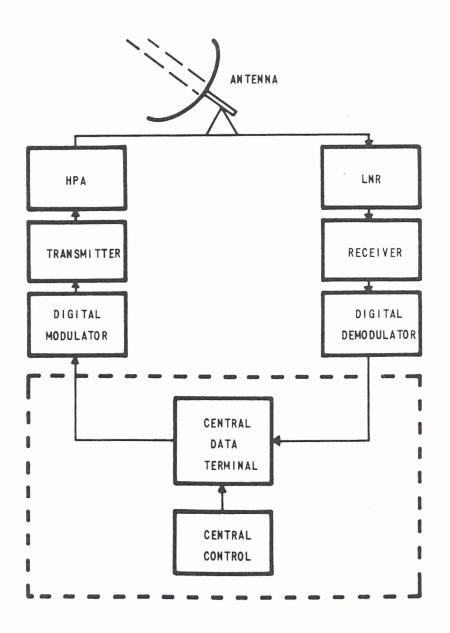
Figure 2-17. Block Diagram of Routing Center
