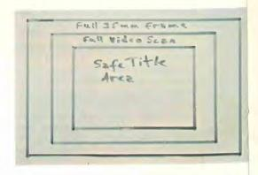
Top and below: a rough field guide is drawn on frosted acetate, lined up with the copy underneath, and the camera is adjusted; then the field guide is pulled off and the copy is shot.
