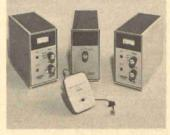
more apart, both receive the transmissions. Both receivers feed a model 62 diversity combiner that selects the receiver with the best signal strength within microseconds. The system is composed of models 54 or 55 transmitter, two model 58 receivers and model 62 diversity combiner.
