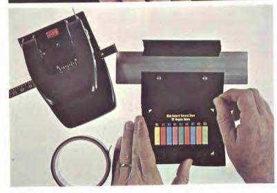
Top to bottom: the author demonstrates opaquing with black masking tape, then using a pin register with the punch.
