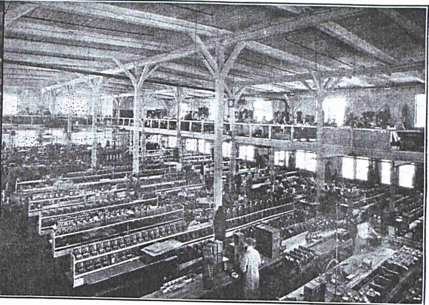
FIG. 6 GENERAL VIEW OF THE MANUFACTURE AND ASSEMBLY OF RC, DA, AND RA SETS
