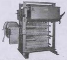
Fig. 58—Controller Equipment for Oil Well Operation with all Arcing Contactors Immersed in Oil.
