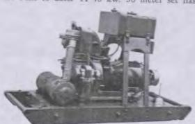
Fig. 64-Portable Radio Generator Driven by Motorcycle Engine.
