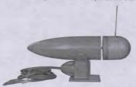
Fig. 65-Wind-Driven Radio Generator for Airplanes.
