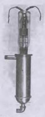
Fig 84-10 kw. vacuum tube with water cooled anode.
